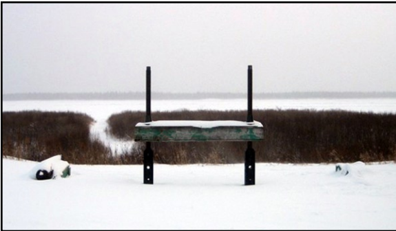
A Beaver Press. These were used to compress the beaver pelts acquired from the Cree by the Hudson's Bay Company. The more that HBC could compress the pelts, the more pelts they got (into the compressed bale) for the fee they paid.
